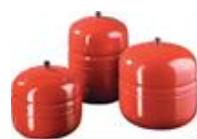
**Expansion vessel:** it absorbs liquid volume variations caused by working temperature variations. In epoxy powder coated steel, long-lasting duration with steady membrane made in SBR rubber. TO ASSEMBLE
