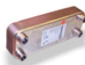
**De-superheaters:** brazed-plate type heat exchanger in steel AISI 316. Based on the recovery water probe temperature, the warm gas is sent in the de-superheater recovering till 25% of condensation heat. The condensation is then completed on the standard condenser increasing the unit performances.
