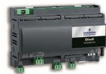
**Control system and remote assistance:** it allows the assistance and the unit remote control by means of PC with web browser. Web server remote connection through corporate network. In case of alarm an alert can be sent via SMS or e-mail. Available in 4 versions:
