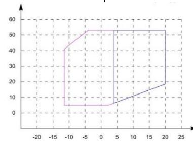
These specific units are designed for high temperature functioning, granting the full running of all the units in condensing till +52°C air temperature.
