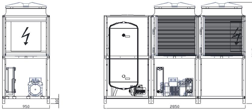
CON KIT IDRICO – WITH HYDRAULIC KIT
