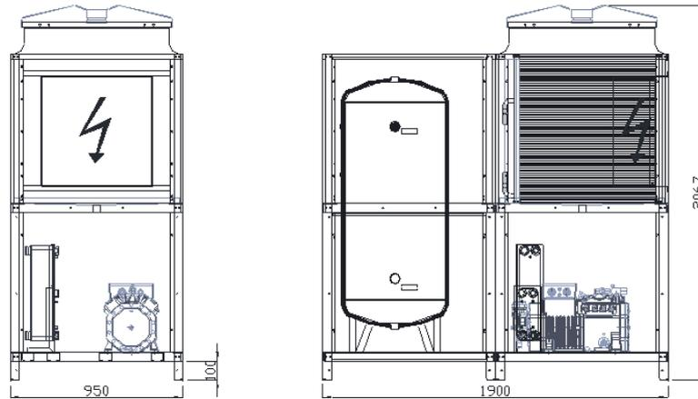
CON KIT IDRICO – WITH HYDRAULIC KIT
