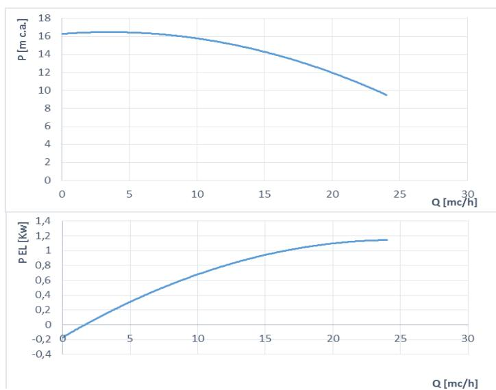
**CARATTERISTICHE TECNICHE****TECHNICAL FEATURES****Pompa – Pump**
