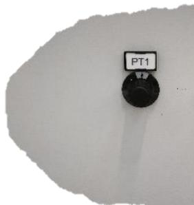
**ATTENTION** For correct operation, the potentiometers should always be positioned on the same value. The air flow adjustment, with ducts installed, must be such that the air flow in / out of the machine is as close as possible with the standard value from the technical data sheet.
