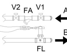
Install the water flow switch FL1 on the outlet hydraulic pipe-line of user water and the contacts connect in the clamps X3-X4 in to the electrical panel, Install the water flow switch FL2 on the outlet hydraulic pipe-line of cold source water and the contacts connect in the clamps X7-X8 in to the electrical panel.
