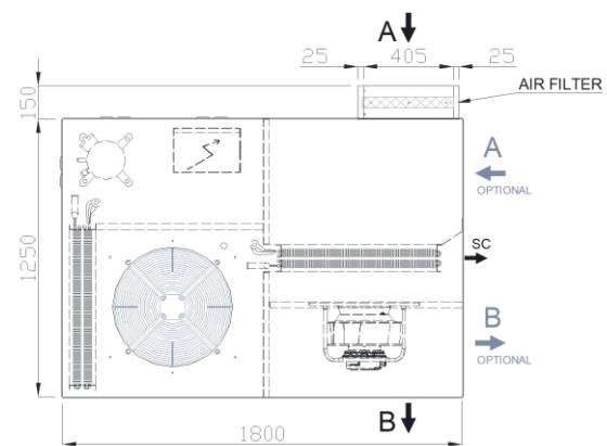
A=INGRESSO ARIA-AIR INLET      B=MANDATA ARIA-EXPULSION AIR      SC=SCARICO CONDENSA-DRAIN DISCHARGE
