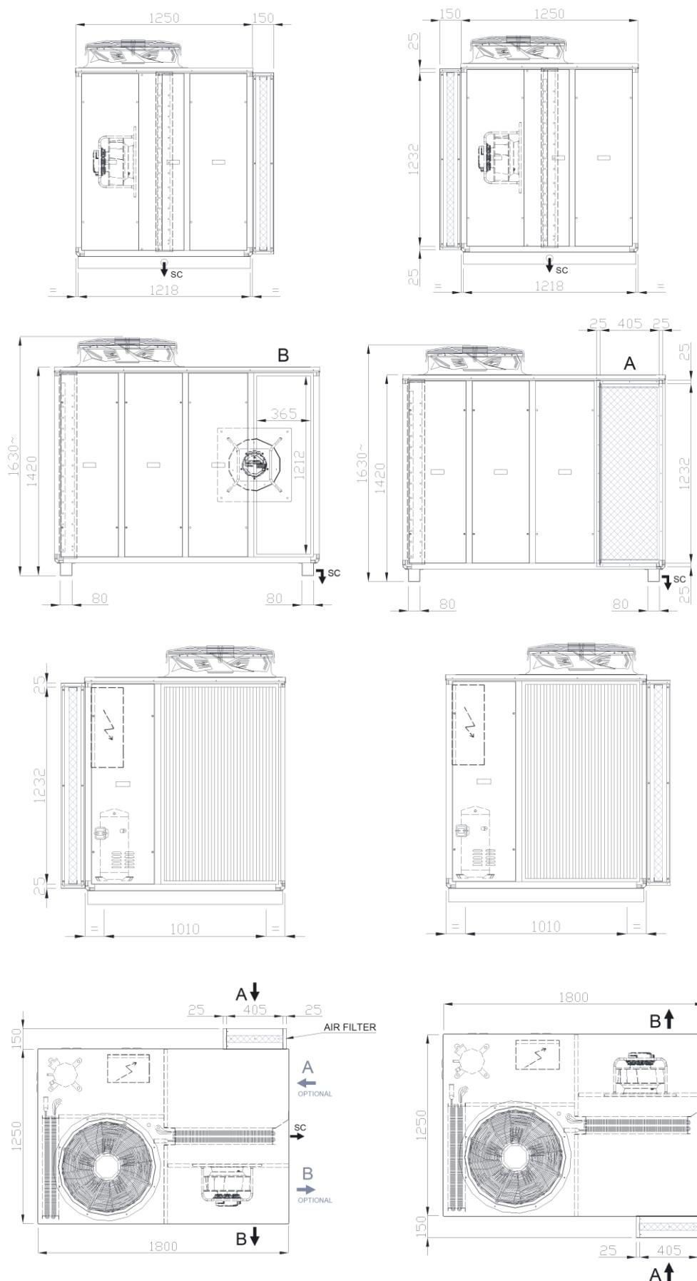
A=INGRESSO ARIA-AIR INLET    B=MANDATA ARIA-EXPULSION AIR    SC=SCARICO CONDENSATION-DRAIN DISCHARGE
