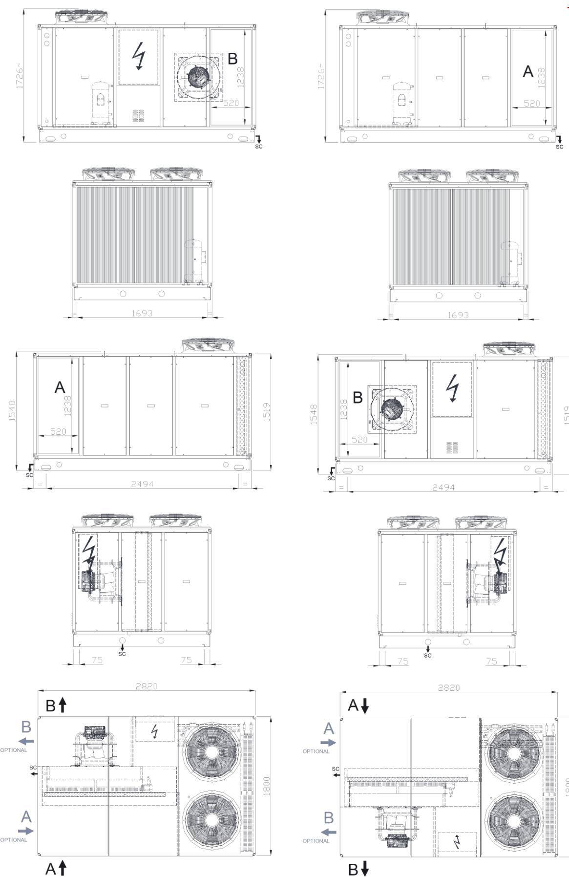
A=INGRESSO ARIA-AIR INLET    B=MANDATA ARIA-EXPULSION AIR    SC=SCARICO CONDENSATION-DRAIN DISCHARGE
