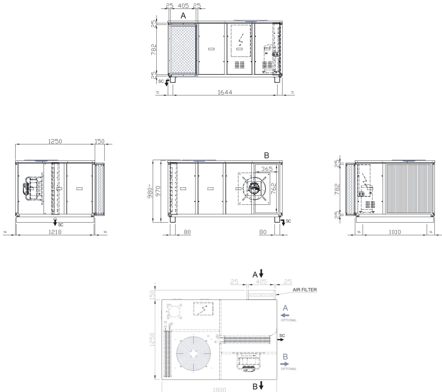
A=INGRESSO ARIA-AIR INLET    B=MANDATA ARIA-EXPULSION AIR    SC=SCARICO CONDENSA-DRAIN DISCHARGE
