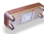
**De-superheaters:** brazed-plate type heat exchanger in steel AISI 316. Depending on the recovery water probe temperature, the warm gas is sent in the de-superheater recovering till 25% of condensation heat. The condensation is therefore completed on the standard condensation by increasing the performances. Suitable for coupling to a fan speed control or EC fans for an unit best use.
