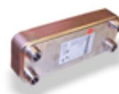
**Total heat recovery:** brazed-plate type heat exchanger in steel AISI. Depending on recovery water probe, the warm gas is sent to the recuperator by giving to the water the condensing energy.
